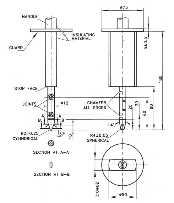
Material — metal, except where otherwise specified. Tolerances on dimensions without specific tolerance:
