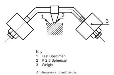
FIG. 5 BALL PRESSURE TEST APPARATUS
