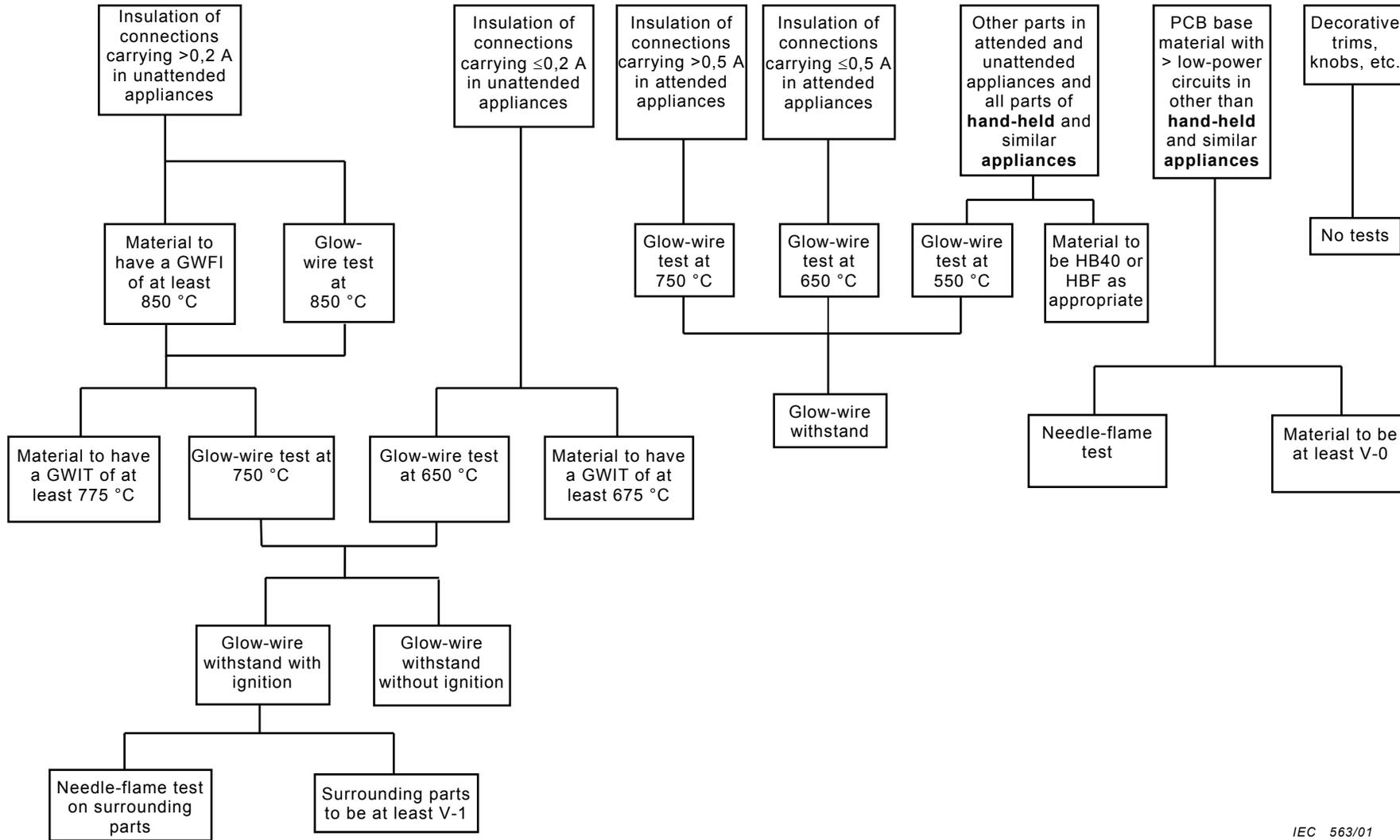
Figure O.2 – Tests for resistance to fire
