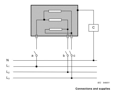
Figure 4 – Circuit diagram for leakage current measurement at operating temperature for three-phase connection of appliances other than those of class II
