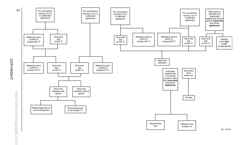
Figure 0.2 - Tests for resistance to fire
