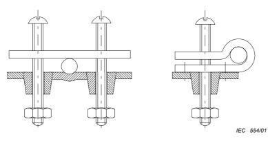
Construction showing part of appliance of insulating material and so shaped that it obviously forms part of a cord clamp.
