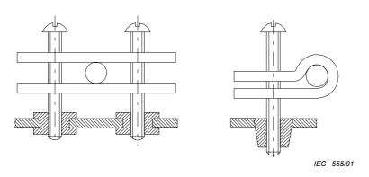
Construction showing no part securely fixed to the appliance.
