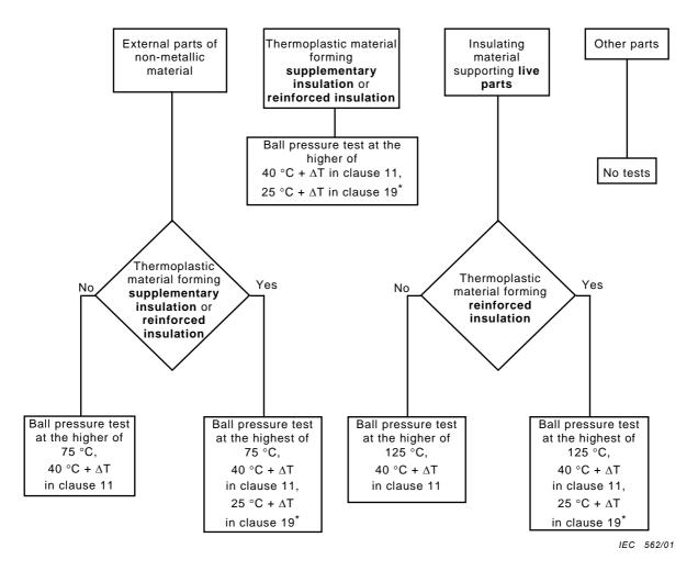
\* $\Delta T$  is not taken into account if the test of 19.4 is terminated by the operation of a **non-self-resetting protective device** requiring the use of a **tool** or removal of a cover to reset it.
