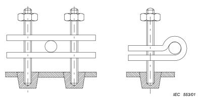
Construction showing studs securely attached to the appliance
