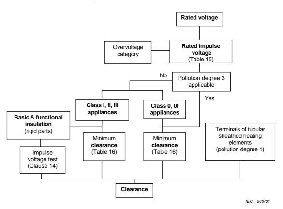
Figure L.1 – Sequence for the determination of clearances
