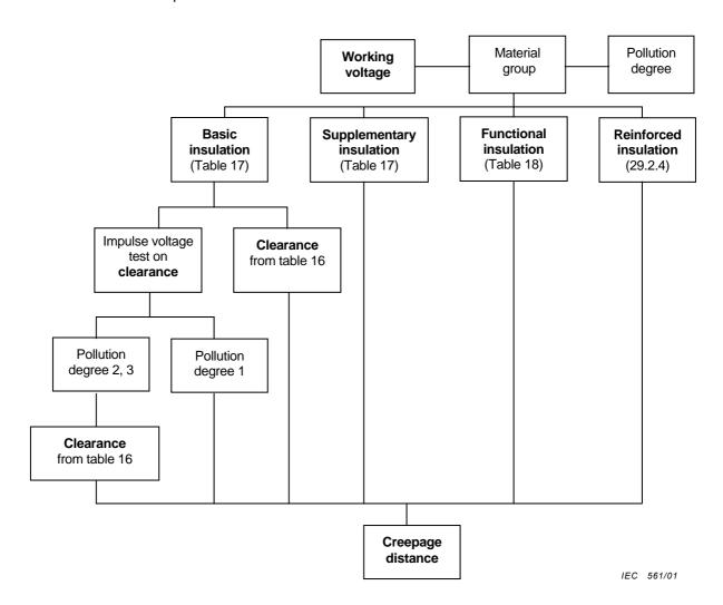
Figure L.2 - Sequence for the determination of creepage distances
