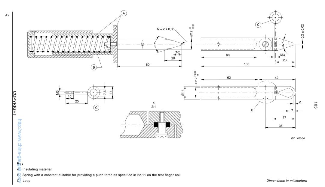
Figure 7 – Test finger nail
