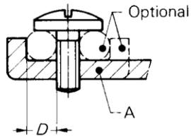
Screw requiring washer, clamping plate or anti-spread device
