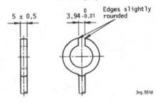
It shall be possible to pass the pin through the "GO" gauge without undue force; it shall not be possible to pass the pin through the gap in the "NOT GO" gauge without undue force.
